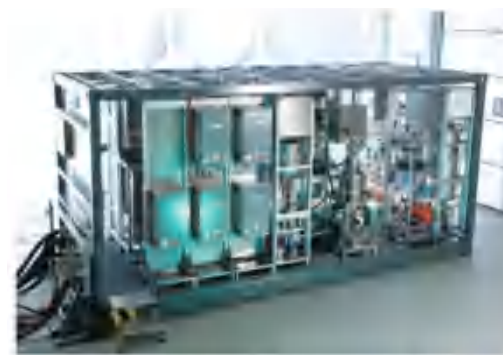
Prefabricated Modular Units Are Increasingly Being Used in the Process and Hybrid Industries (Source: INVITE GmbH, Leverkusen)
